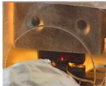
temperature measurement at initiation of necking
