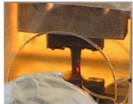
temperature measurement post necking
