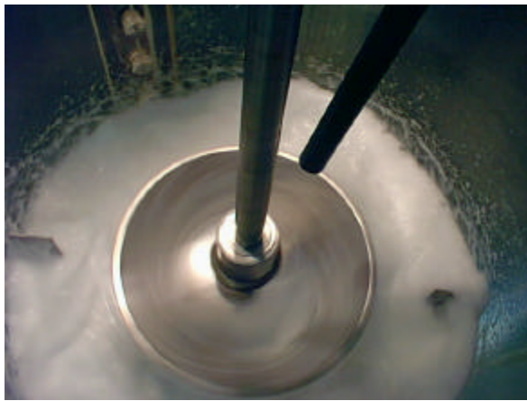
Figure 15: 0.61m vessel, 274 rpm, and 10 ppm soap. Level completely under control
