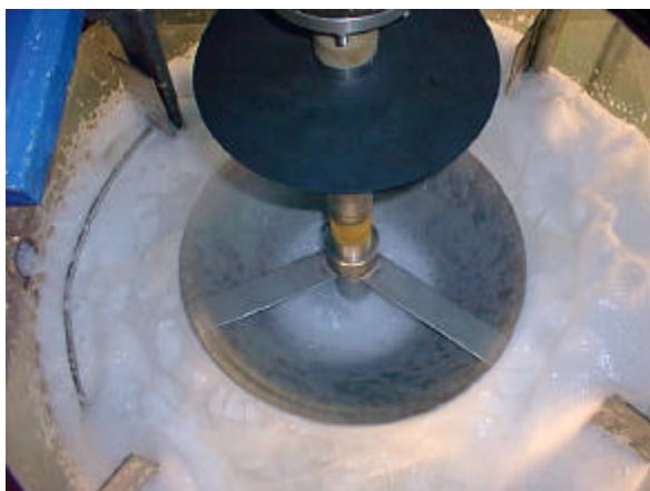
Figure 17: 0.914m vessel. Reducing foam at 180 rpm after complete foam-out at 40 rpm.
