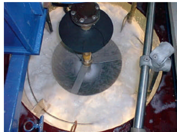
Figure 18: 0.914m vessel. Equilibrium foam at 180 rpm.
