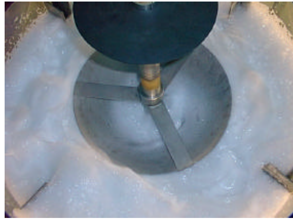
Figure 20: 0.914m vessel. Just coping with foam at 140 rpm
