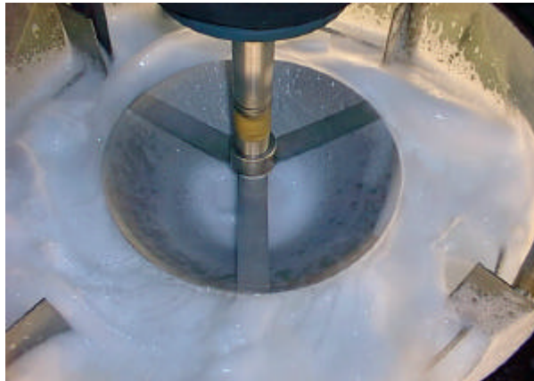
Figure 19: 0.914m vessel. Stable operation at 150 rpm
