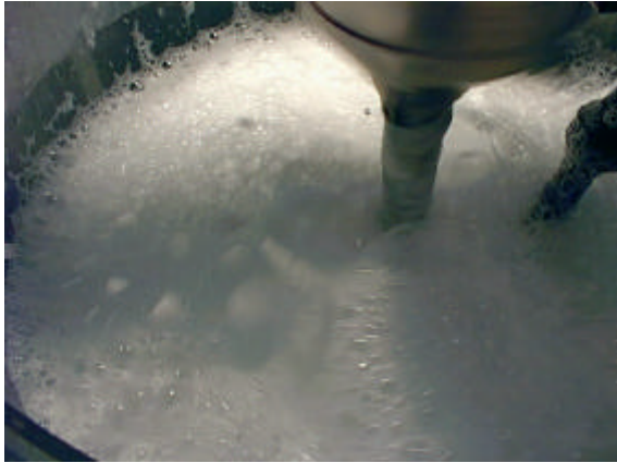
Figure 13: 0.61m vessel. Cone flooded, agitator switched on to bring foam under control. 10 ppm soap
